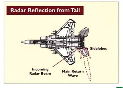
of LO design. A large, flat plate reflects radar return like a mirror. Conventional aircraft with large vertical stabilizers are textbook examples.
