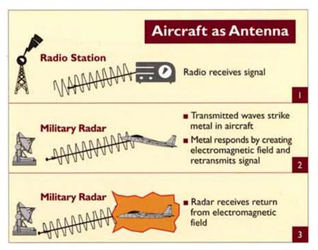
These currents then create new electromagnetic waves, depicted in Panel 3, that are emitted from the aircraft in various directions and, depending on where they strike the aircraft, are seen by the radar receiver as reflected echoes. These echoes are significantly weaker than the original electromagnetic waves transmitted by the radar.
