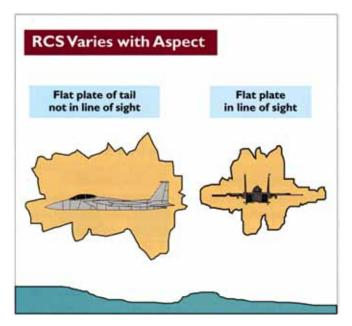
the intake walls and from diffraction inside the cockpit area. Waves will travel along the wings until they are diffracted from the wing tips and returned from the trailing edge. From the side, the RCS will be much larger. The flat plate of the vertical stabilizer presents a large specular reflection, plus corner and edge diffraction. Pods, ordnance, or drop tanks under the wings will also cause larger returns.
