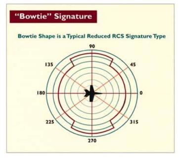
reduce radar cross section and improve survivability. Applying radar-absorbing material to forward surfaces, shielding inlets, ducts and canopies, and minimizing ordnance and other protrusions are some of the measures that can lower RCS from the nose-on angle. Rear and side aspects would not be reduced in the same way. Thus, in this notional case, a retrofitted aircraft might have a signature reminiscent of the creature in the old 1970s Pacman video game.
